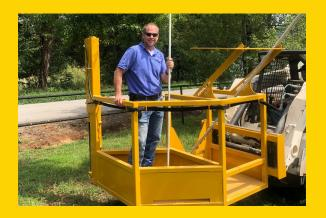
The BIG JOHN Gopher is designed to minimize the time and cost of staking large quantities of trees. Rather than climbing a ladder and hand driving stakes in, the Gopher's hydraulic stake drives into the ground to make holes for the trees. The Gopher allows you to carry multiple stakes in the hopper and place in the trees as you go.
