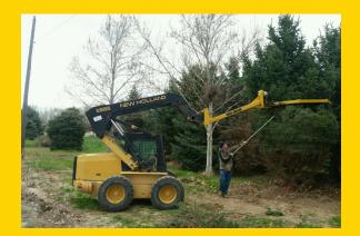
The BIG JOHN Limb Lifter is designed to minimize time and cost of typing 3" to 12" trees. Easily mount it to your skid steer or other power units to tie up your trees in minutes. It's wide, adjustable, has a 6-foot opening and large 2.5" x 32" rollers that lets you tie up larger trees while preventing limb damage.
